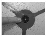
If the disc does not rotate freely, turn the disc over. On the underside of the disc at the center of the base plate, there is a retaining cap with drain that retains the end of the recovery line with the shear washer. Flush the retaining cap with clean water to clear any internal debris and re-test to insure that the disc rotates freely. Insure that the retaining cap is intact.
